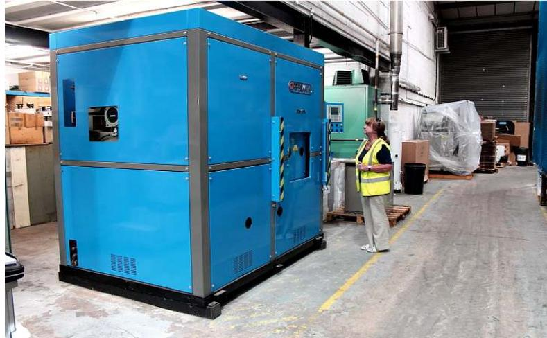
*A Fibimatic sealed vapour degreasing machine, supplied by Standard Industrial Cleaning Systems. Glenn Greenlees says that Environmental Health Officers generally only have experience of "open top" tank degreasing systems and have little or no knowledge of modern technology such as the machine pictured here.*
